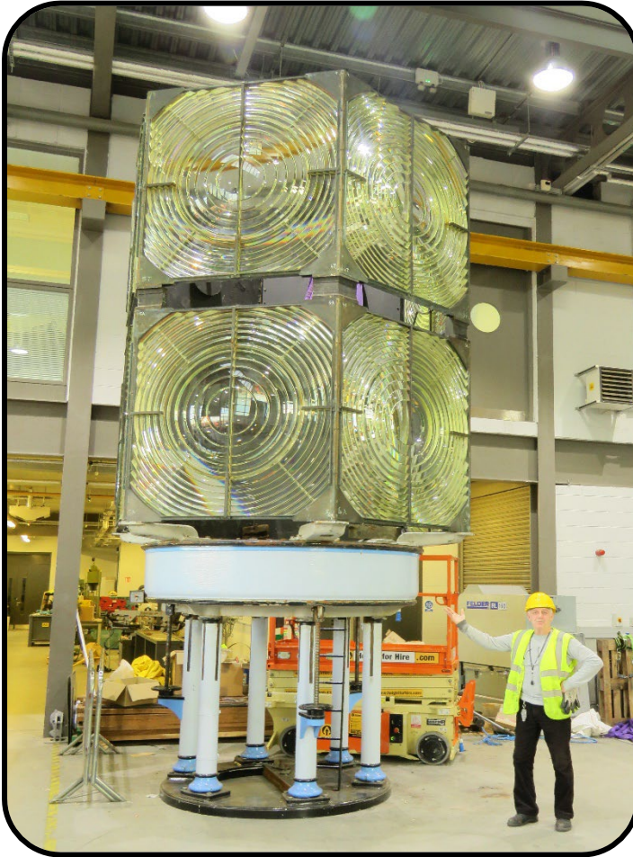
Figure 3: Hyper-radial Fresnel lens and pedestal
