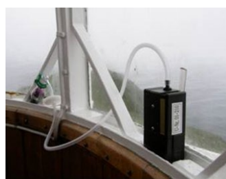
Figure 10: Tabel shows different contamination levels and at right an arrangement for measuring mercury concentrations in air.
