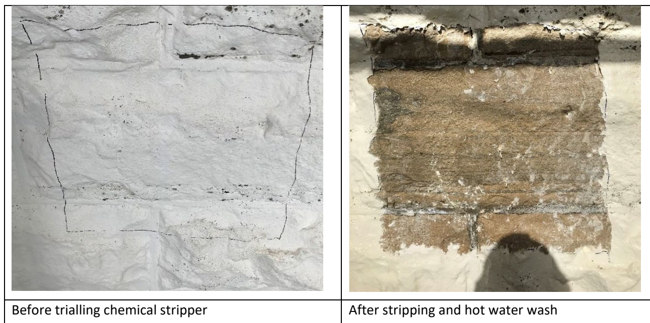
Figure 4: Paint removal to stone
