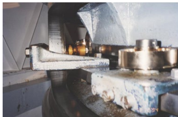
Figure 1: Revolving optic system with roller carriage – at right details from a roller carriage system.
